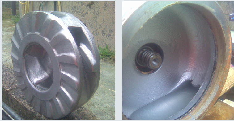
Figure 7a. Even wear on WBH® impeller
