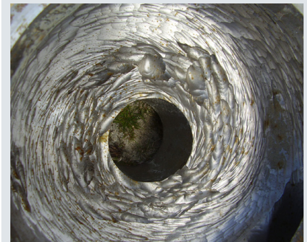
Figure 6a. 4/3 AH ® throatbush at 2,200 hours (no adjustment)
