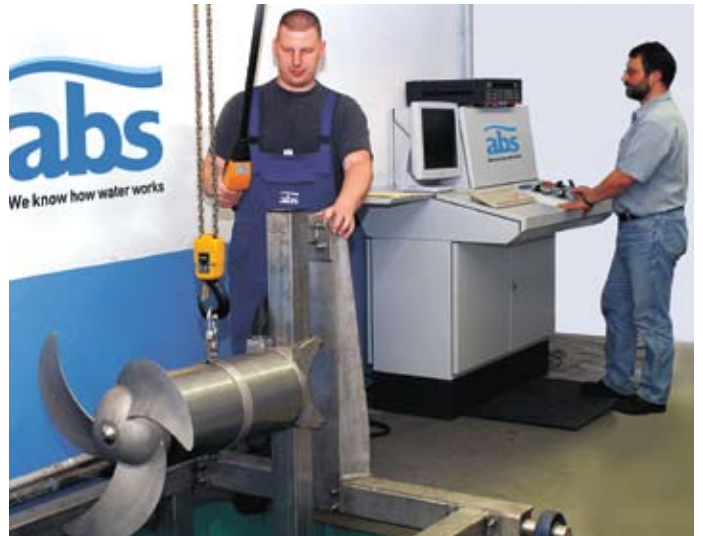
Thrust measurement facility regarding ISO 21630.
